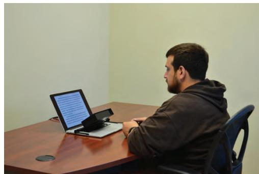
The EyeLink Portable Duo includes adjustable Tripod and Laptop Mounts to enable superior quality eye tracking data collection in a wide variety of settings, both in and out of the laboratory.
