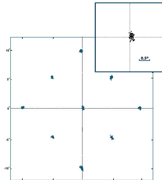
Repeated target fixations to nine screen locations recorded with the EyeLink Portable Duo with the head stabilized following a 13-point calibration. The inset plot represents an enlarged view of the fixation distribution around the center target position. On the right is a fixation error histogram demonstrating the tight fixation accuracy distribution (Mean = 0.25°, Median = 0.23°, and Standard Deviation = 0.14°).
