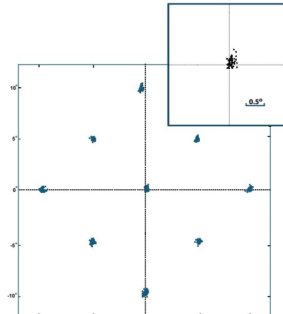
Accuracy was assessed without a head support using the Remote Mode following a 13-point calibration. Repeated target fixations to nine screen locations resulted in the low error levels demonstrated by the fixation error histogram below (Mean = 0.26°, Median = 0.22° and Standard Deviation = 0.16°). The inset plot is an enlarged view of the fixation distribution around the center target position.
